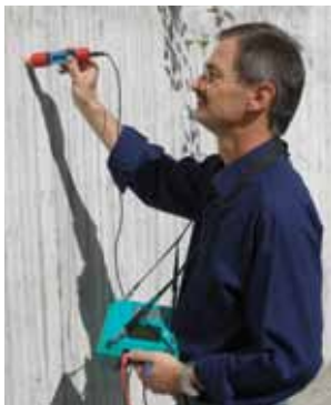
Standard Copper / Copper Sulphate Rod Electrode for localized measurements
