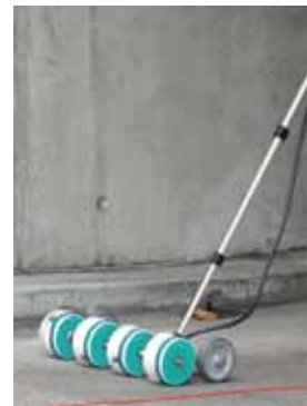
4-Wheel Electrode for maximum measurement speed on large areas
