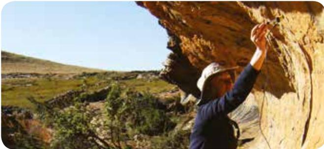
Extensively used for rock hardness and for investigating weathering effects on rocks. The impact energy is approximately 1/200th that of the Type N rebound hammer.
