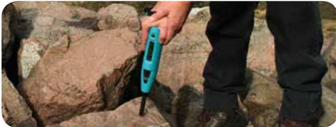
The world's most advanced rebound hammer, with unmatched dispersion characteristics, durability and measuring range has now been fully adapted for rock testing. The following features of the hammer make it ideal for rock testing applications:
